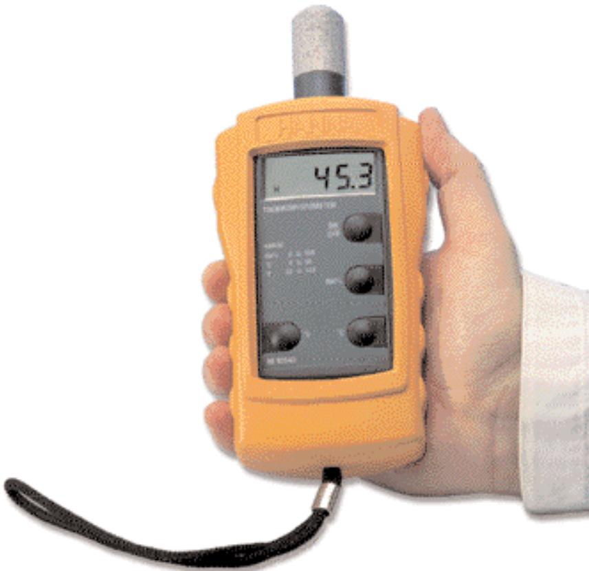
HI 93640 is a compact, portable and versatile hygrometer to monitor relative humidity anywhere.
